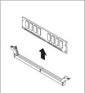
Figure 10. Removing the memory module
